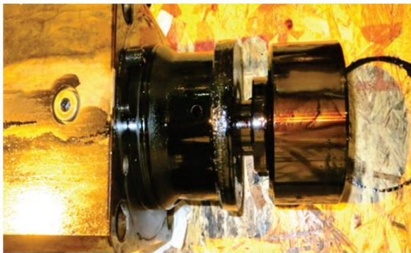
Fuel booster plunger stuck in the barrel
